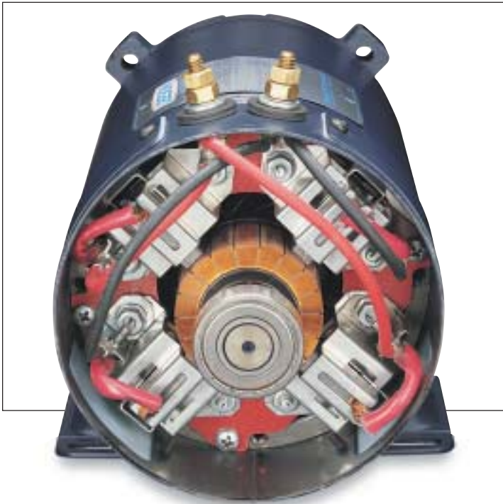
NEMA and IEC frame DC motors from LEESON feature oversized brushes, accessible without disassembly of the motor. Integral constant pressure springs and bi-directional brush holders help ensure long service before maintenance — up to four times that of other DC motors. Four brushes are used in larger horsepower low voltage motors.
